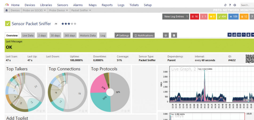
figure 3 : Analyzing connections via packet sniffer
